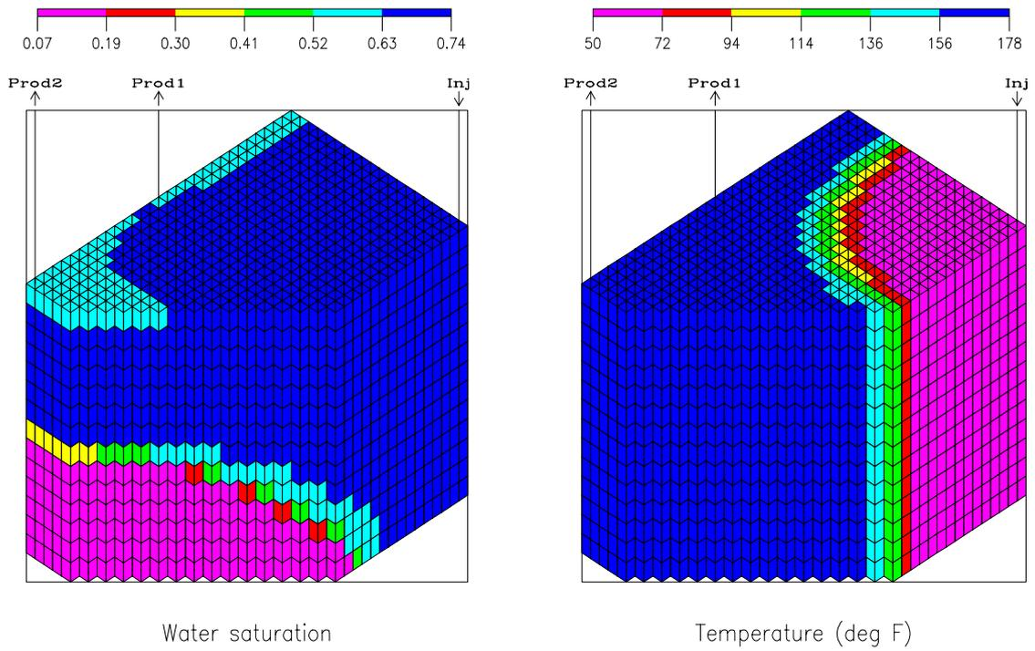
**Figure 9: Water and temperature distribution at start of treatment (3000 days) in thin layer model**
