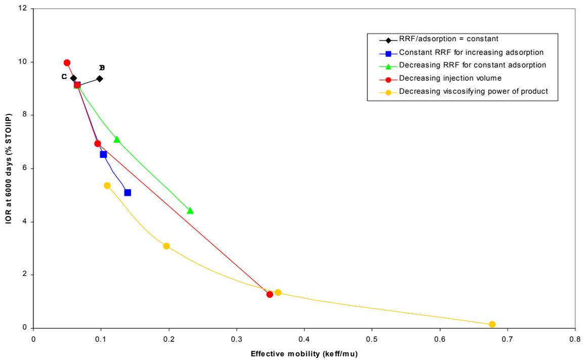
Figure 7: IOR vs. final effective mobility for treatments in thick layer model with sealing barrier between layers
