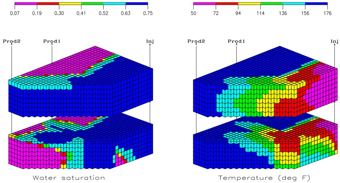
**Figure 14: Water and temperature distributions at start of treatment (3000 days) in two channel model**
