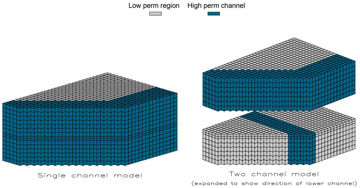
**Figure 12: Schematic of channel sands models**
