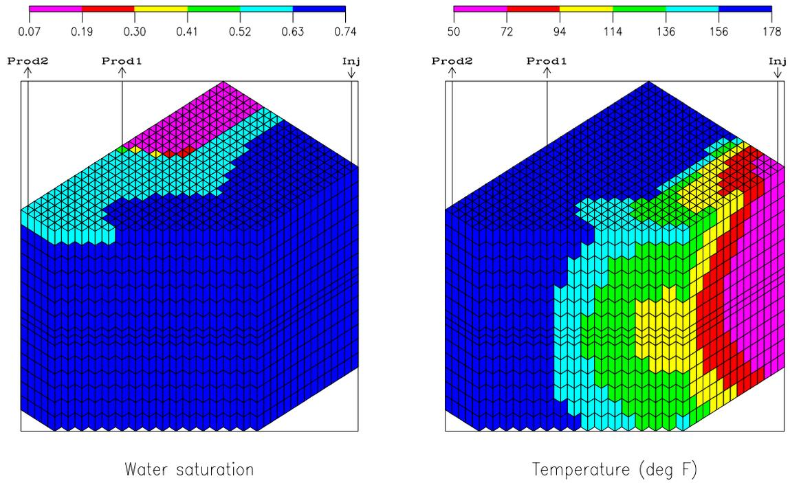
**Figure 13: Water and temperature distributions at start of treatment (3000 days) in single channel model**
