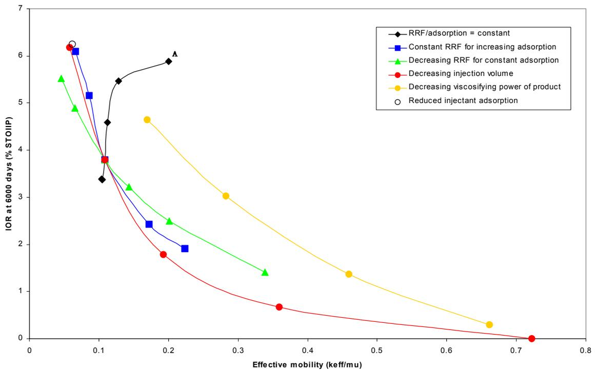
**Figure 5: IOR vs. final effective mobility for base case thick layer model treatments**
