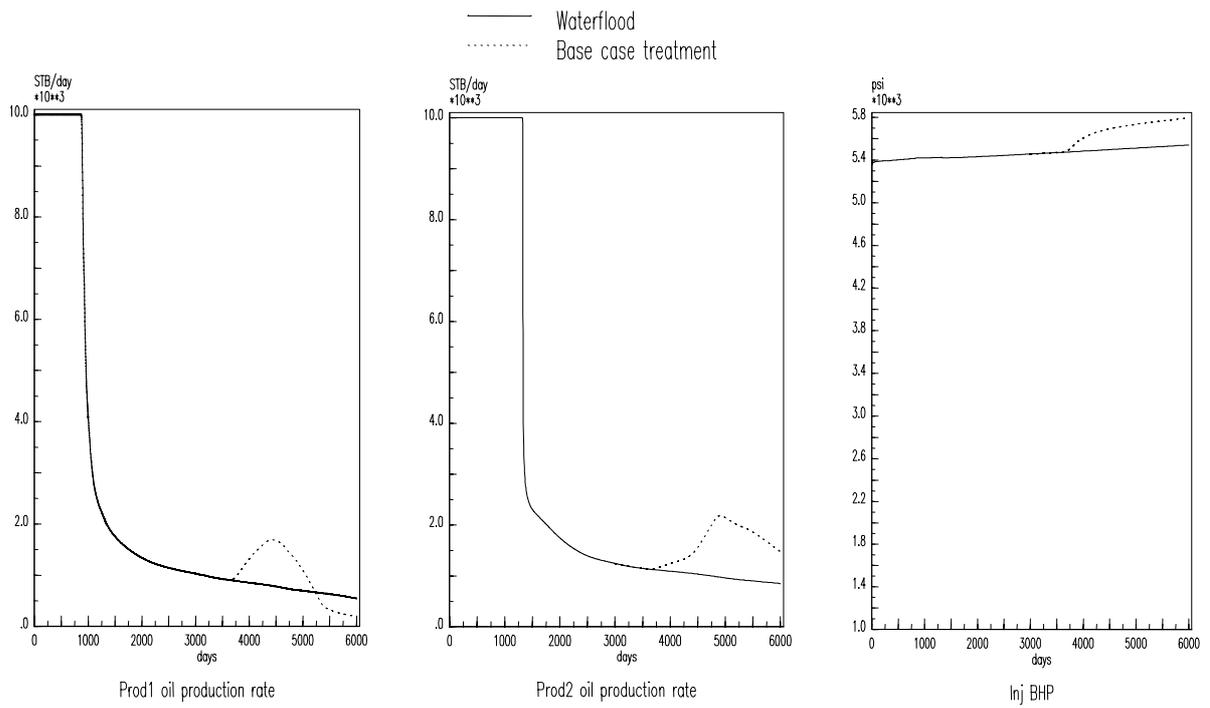
**Figure 3: Oil production profiles and injector BHP for thick layer model waterflood and base case treatment**
