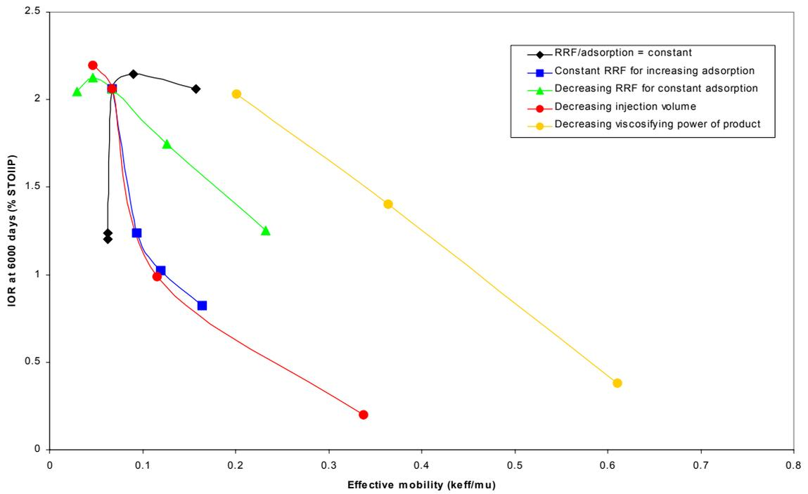
Figure 6: IOR vs. final effective mobility for treatments in thick layer model with increased vertical permeability
