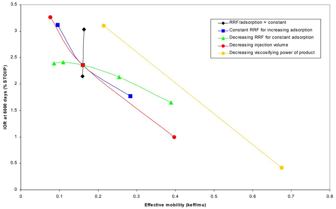
Figure 10: IOR vs. final effective mobility for treatments in thin layer model
