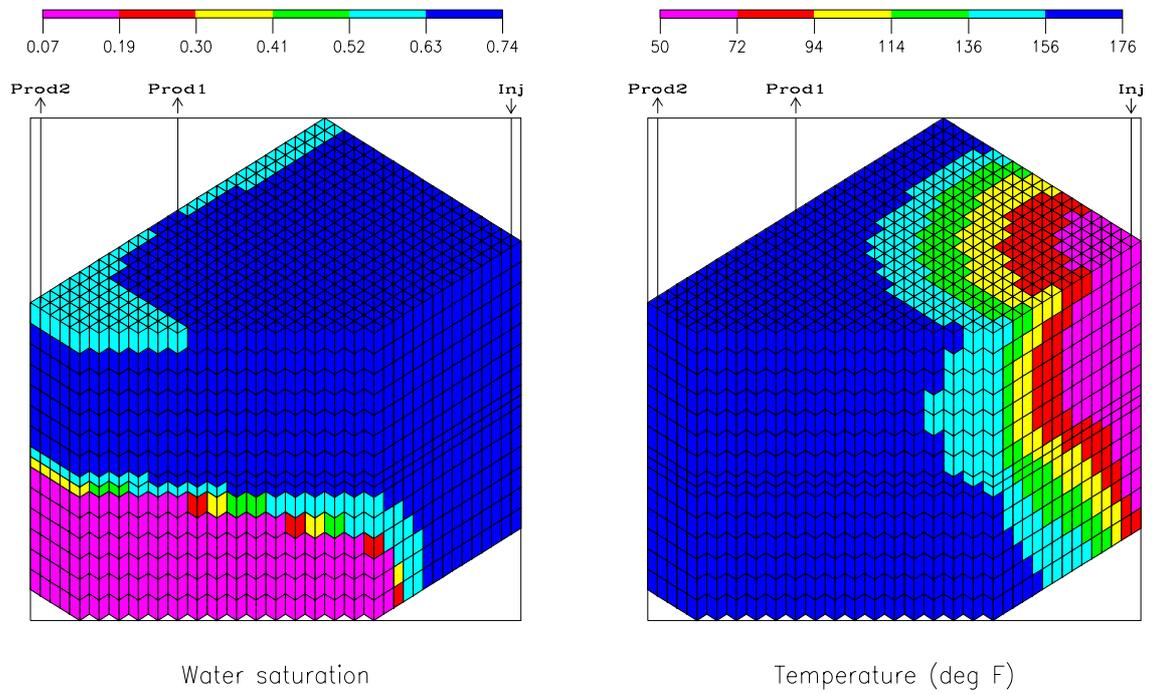
**Figure 2: Temperature and water distributions at start of treatment (3000 days) in base case thick layer model**
