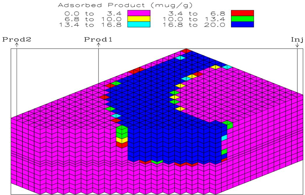
**Figure 4: Final placement of mobility reducing agent in thick layer model base case treatment**
