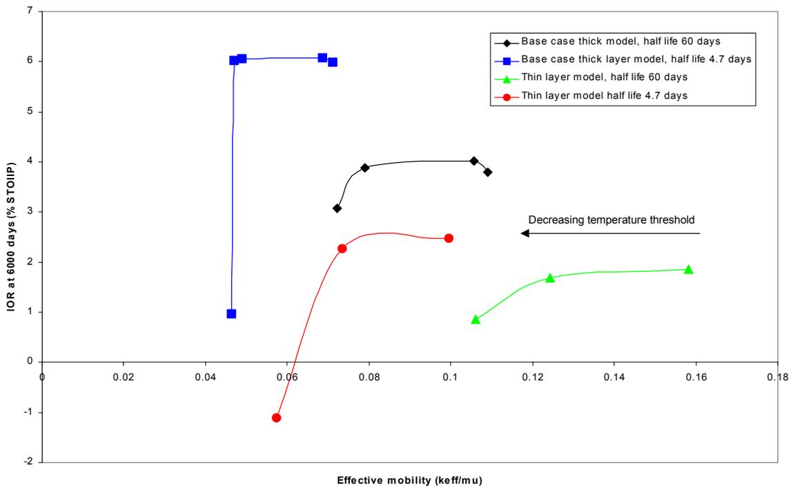
Figure 11: IOR vs. final effective mobility for treatments varying reaction temperature threshold
