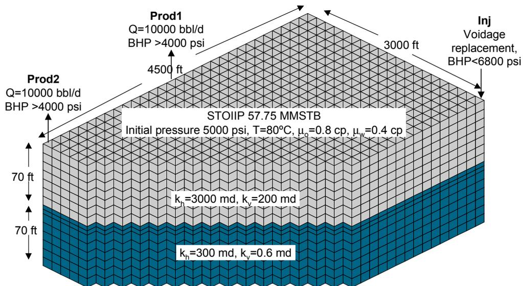
Figure 1: Schematic of base case thick layer 'Etive-Rannoch' model
