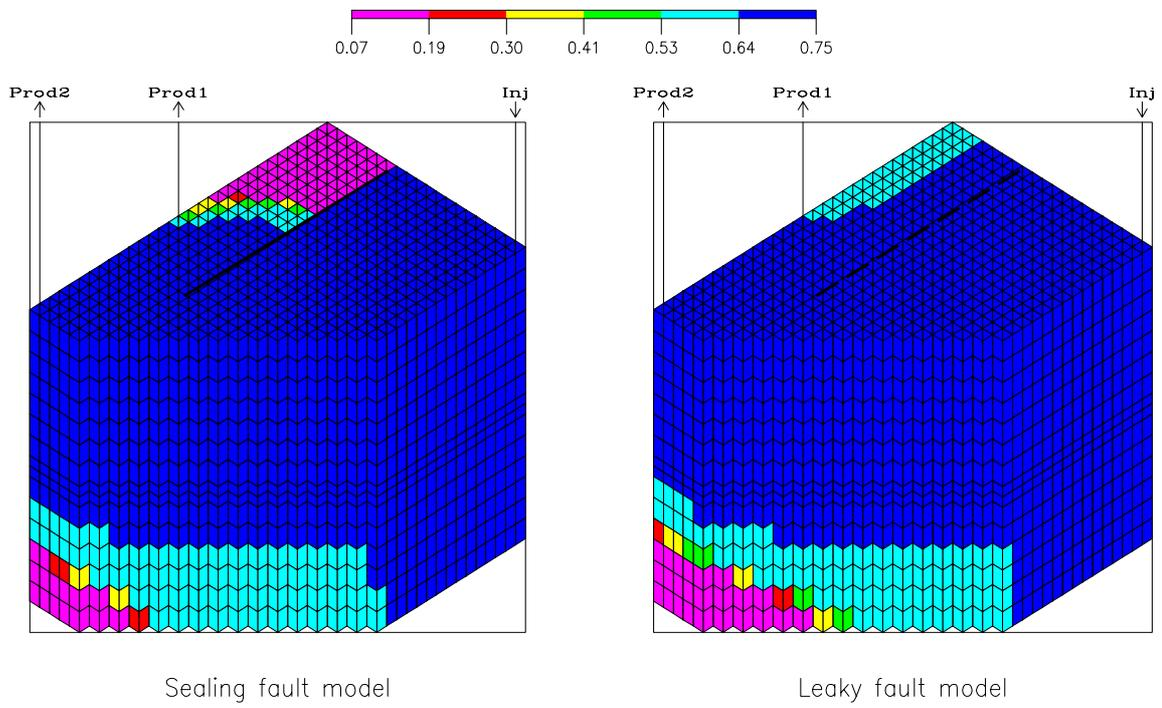
**Figure 8: Final water saturations in thick layered models with sealing and leaky faults**
